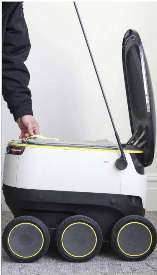
The robots from Starship Technologies have removable linings to keep the delivery items they are carrying at the appropriate temperature.
