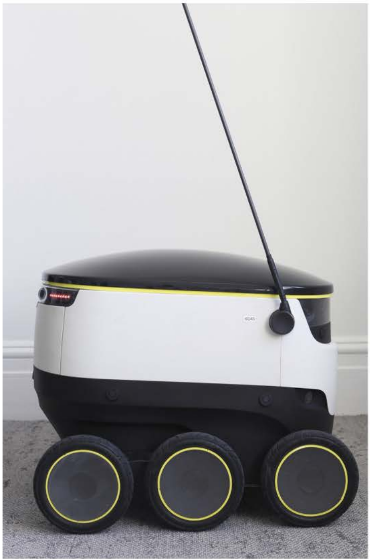
The robots from Starship Technologies have removable linings to keep the delivery items they are carrying at the appropriate temperature.
